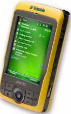
The integrated GPS receiver provides accurate positioning information within 5 meters when using real-time or postprocessed differential correction. For more information, see Chapter 5, Using the GPS Receiver.
