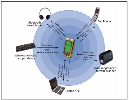
Figure 7.1 Juno series handheld Bluetooth client connections
