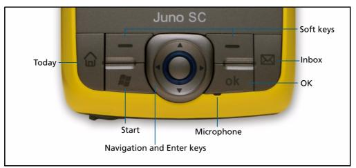
Figure 2.4 Juno series handheld keypad buttons
