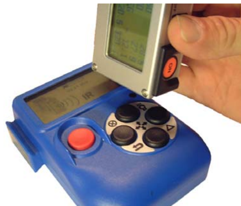
Ex. Sending data to the Digitech Professional caliper
